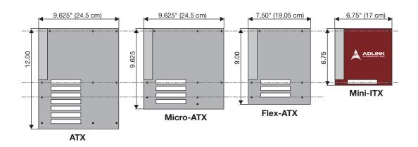
In addition to deployment in smaller chassis designed around the Mini-ITX form factor, these boards are compatible with ATX and microATX chassis without the need to retool the I/O shield. Mini-ITX boards are ideal for applications in industrial automation, self-service kiosks, and other infotainment driven solutions.
