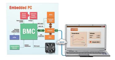
Interfacing the hardware to the operating system is one of SEMA's most important functions. The BMC first collects all relevant information from the chipset and other sources. Using the System Management Bus driver, the application layer fetches the data and presents it to the user.
